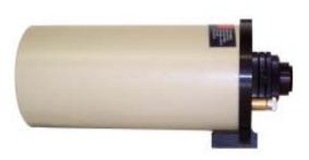
The newly designed low profile mount has strengthened the overall package while adding two basic built-in zero power sight mechanisms. The new single-piece aluminum tube construction together with the Questar integrated lens cell increase the ruggedness and hold the optical alignment under extreme conditions. The rear backplate assembly has also been improved to increase ruggedness and reduce weight.
